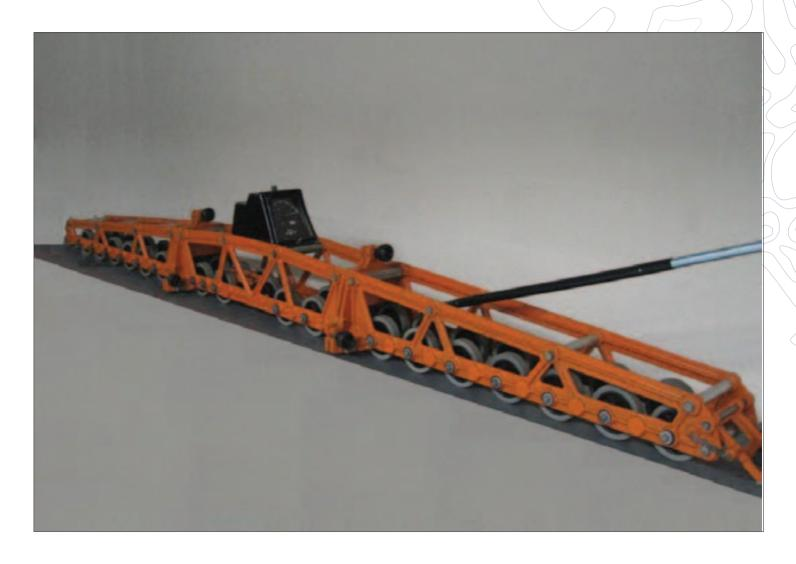
The Rolling Straightedge measures depressions on the pavement surface on analogue scale 0-12mm + 0.25mm. The straightedge also has an odometer for accurate determination of distance travelled in units of 1 metre.
