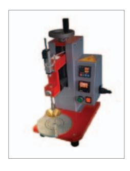
The Semi Automatic and Full automatic Penetrometer gives you better control when used to determine the penetration of bituminous samples. It comes with build in digital controler and readout unit. During the test, depth penetration is permanently displayed both in units and tenth of units (0.01 mm). An optoelectronic detection of depth penetration with an automated approach and a levelling system for conductive samples are available.
