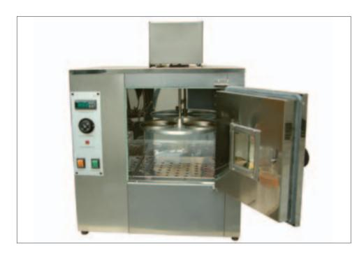
The Loss on Heat Oven test method is used for determining the loss in mass, the effect of heat and air on
