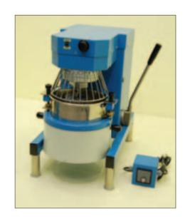
The Isomantle Heater is Used to heat the mixing bowl of (5 litres cap.) and (10 litres cap.) mixer.
