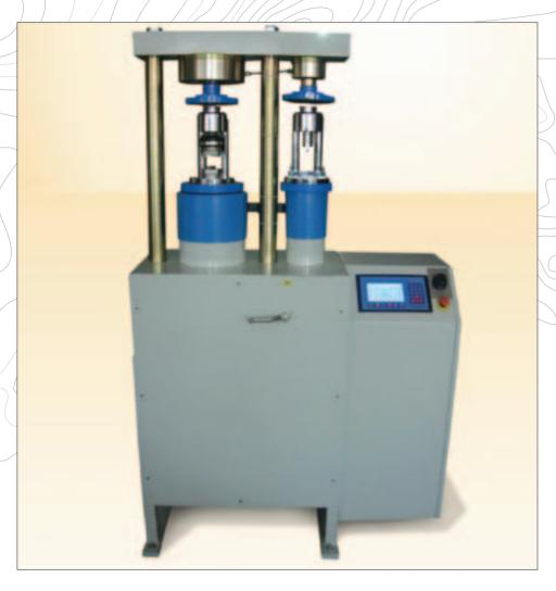
The Cement Compression and Flexural Machine 25/250 KN is Fully Automatic and has been designed for testing the compression on the 50x50x50 mm cube moulds, 40x40mm and the flexural on the 40.1x40 x160 mm prism moulds according to the related standards.
