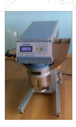
Automatic Digital Mortar Mixer is perfect to mix mortars and cement material according to the required standards.
