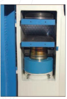
The Block Test Platens 510mmx310mmx50mm are used for testing concrete blocks and other structural materials.
