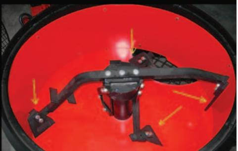
The Planetary Concrete Pan Mixer is efficient for mixing concrete samples for laboratory.
