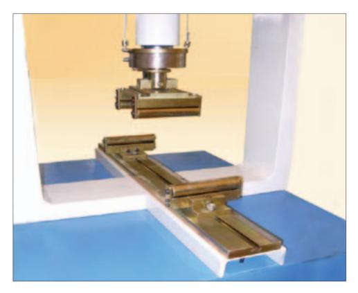
The Flexural Test assembly on Concrete Beams is used for 3 or 4 point flexural tests on 100 or 150 mm concrete beams.
