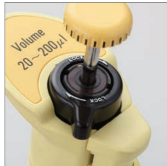
Easy calibration with enclosed jig
